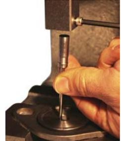
3. Place the Shell Plate flat side down into the alignment flange on the reloading press. Place a fired casing into the Shell Plate with the propelling
