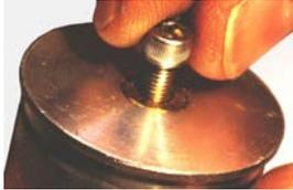
c. Take the additional 10-32 stainless set screw and screw in by hand until flush.
