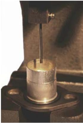
charge down. Carefully bring the ram down by slowly turning the handle. Make sure the extraction pin is not bent and goes easily into the flash-hole of the casing. Just inside the flash-hole, the pin will make contact with the fired propelling charge. Use firm, steady pressure on the ram handle to extract the spent cartridge
