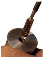
7. Clean propelling charge hole with a .40 caliber brush (not included) to ensure that it is clean and free of debris. **DO NOT** use solvent to clean the hole, as this may damage the casings.
