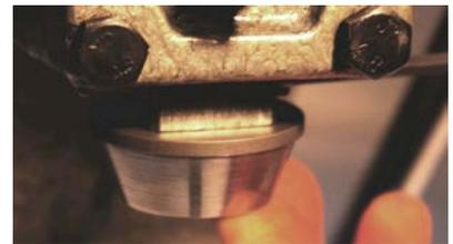
3. Use the wax lubricant stick to apply a thin line of lube around the beveled face of the TX-40™ Expander Die.
