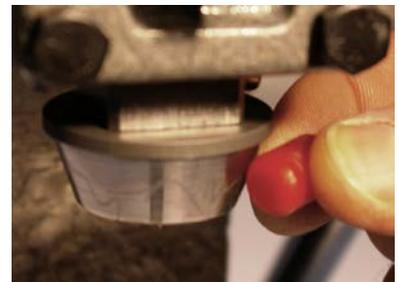
4. Place the Shell Plate flat side up into the alignment flange on the reloading press.
