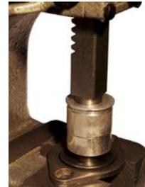
5. Bring the ram down to the base of the empty casing.
