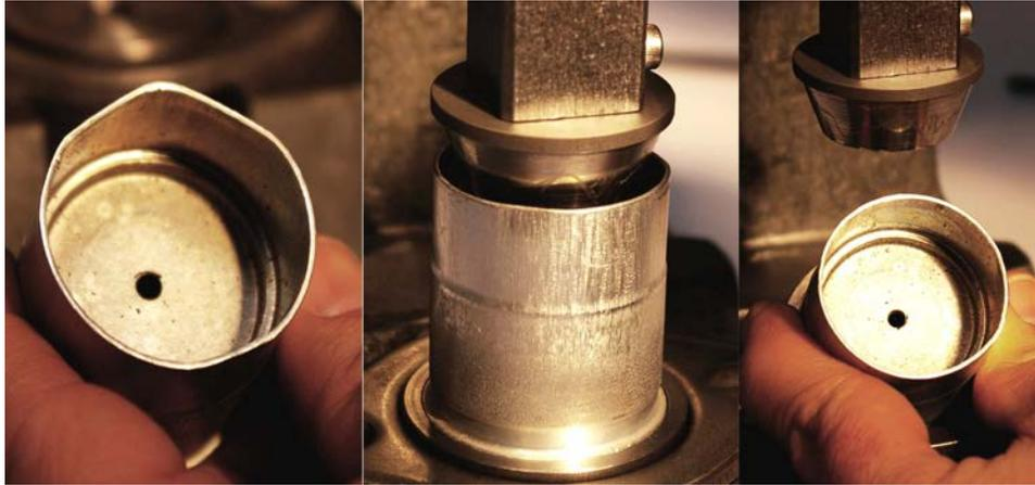
Steps for using the TX-40 Expander Die to repair dented case mouths:
