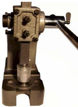
11. Place the casing on the Propelling Charge Seating Block so that the protruding cartridge is on top. Carefully bring the ram down by slowly turning the handle to bring the seating punch into contact with the propelling charge. Use firm, steady pressure on the ram handle to seat the new cartridge flush to the casing (this may require some effort).
