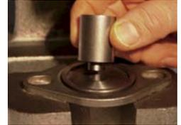
3. Insert the Propelling Charge Seating Block into the shell plate. There is a nipple on one end that goes through the hole in the shell plate.
