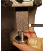
2. Insert the Propelling Charge Seating Punch fully into the ram, and hand-tighten the set screw to hold the seating punch in place.
