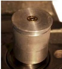
If propelling charge will not seat perfectly flush, try loading the shell into the launcher to assure that the breach will fully close. The propelling charge does not have to be perfectly flush, it simply needs to chamber and allow for the breach to close.
