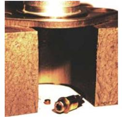
5. DefTech casings often have a brass burst cup pressed into the propelling charge hole. **Remove it before reloading!** To remove, use a Letter T drill bit (not included) at a very low speed with light pressure to grab the cup. Pull it out as the drill bit spins.
