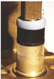
to seat the projectile with the Reloading Press. To do this, remove the seating block from the Shell Plate and place the primed casing into the Shell Holder. Align the projectile with the case mouth and bring the ram down by turning the handle. The seating punch will provide even pressure to seat the projectile. This results in a fully reloaded cartridge.
