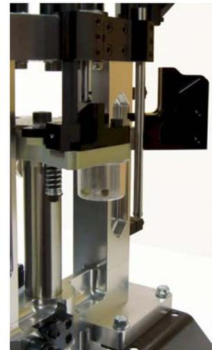
If the LRP (large rifle primer) system is being used, then the LRP Primer Tube Insert Assembly must be installed, along with the LRP Primer Shuttle. The LRP tube is designed to hold up to 100 large rifle primers. Standard large primer pickup tubes or automated primers fillers can be used to fill the LRP tube.
