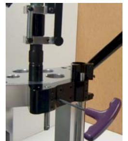
powder die funnel. Continue to pull the handle down until either the handle reaches the bottom of the stroke or the powder measure runs up to the top. Adjust the powder die up or down (by turning the whole powder measure and powder die together) until you reach the bottom of the stroke of the handle at the same time as the powder measure handle runs up to the top of the powder measure. Lightly tighten the nylon set screw to lock the position. Very little force is needed here.
