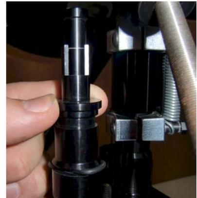
7. Insert the correct Powder Check Probe (caliber specific) into the top of the Powder Check Adapter. Rotate the adapter until the window cutout is facing the front.
