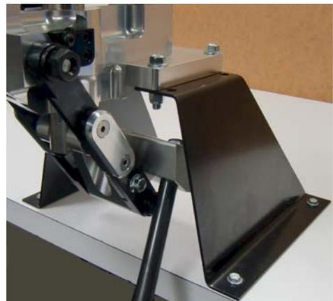
3. Now, measure out 11-3/4" to the right from the center of the front left bench stand hole marking across the front edge of the bench and make a mark. Then, measure back from the front edge of the bench the distance of the measurement you took in number 2 above, and make a mark. This mark will represent the center of the front right bench stand hole.
