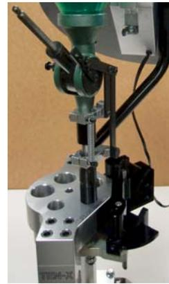
6. After the Powder Die height is correctly set, the Powder Check die can be installed. The Powder Check Adapter is attached to this die and is supposed to be free-spinning. Carefully thread the die into the Head Plate in the 1" hole next to the installed Powder Die. Do not insert this die too deeply and do not tighten the nylon set screw until final adjustments are made with a casing filled with the desired powder charge.
