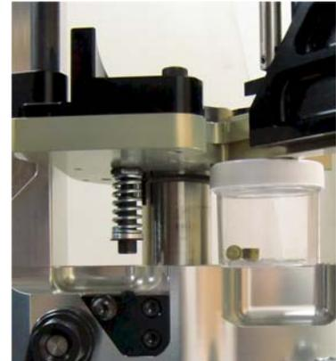
The second function of Station Two is performed when the handle is pulled down to raise the platform and a case is positioned in Station Two. The case activated RCBS Powder Measure will dispense the charge that has been set. The powder drop will need to be adjusted to the desired powder weight. It is important to use a quality powder scale to do this.
