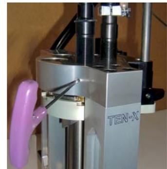
10. When the desired position of the line is where you want it, lightly turn the nylon set screw on the left side of the Head Plate to lock the die. Never over-tighten the set screw as it can easily be stripped. Very little pressure is needed to lock the die in place.
