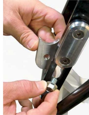
**NOTE:** If your TX-50™ has the collapsible link arms installed and you are not priming, it is strongly recommended you reattach the Link Arm Lock to the link arm nearest the handle. This will ensure a smoother loading process, a shorter stroke, and reduced wear on the press.
