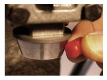
4. Place the Shell Plate flat side up into the alignment flange on the reloading press.
