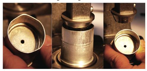
Steps for using the TX-40 Expander Die to repair dented case mouths:
