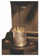
charge down. Carefully bring the ram down by slowly turning the handle. Make sure the extraction pin is not bent and goes easily into the flashhole of the casing. Just inside the flash-hole, the pin will make contact with the fired propelling charge. Use firm, steady pressure on the ram handle to extract the spent cartridge
