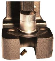
(this may require some effort). It may be necessary to bring the ram up and then down a second time to release the spent propelling charge from the casing. Recycle or discard the spent charges and burst disks (if any) that collect in the space under the press.
