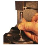
3. Place the Shell Plate flat side down into the alignment flange on the reloading press. Place a fired casing into the Shell Plate with the propelling
