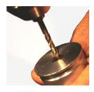
a. Drill out the brass primer pocket of the stuck propelling charge with the #18 drill bit. [If you are reloading a CTS casing, a #24 drill bit is required to open the flash hole of the metal insert from the inside of the plastic casing.]
