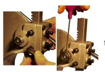
8. Replace the crank handle retaining ring and tighten the set screw.
