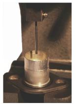
charge down. Carefully bring the ram down by slowly turning the handle. Make sure the extraction pin is not bent and goes easily into the flashhole of the casing. Just inside the flash-hole, the pin will make contact with the fired propelling charge. Use firm, steady pressure on the ram handle to extract the spent cartridge
