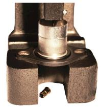
(this may require some effort). It may be necessary to bring the ram up and then down a second time to release the spent propelling charge from the casing. Recycle or discard the spent charges and burst disks (if any) that collect in the space under the press.
