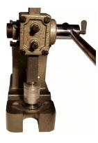
11. Place the casing on the Propelling Charge Seating Block so that the protruding cartridge is on top. Carefully bring the ram down by slowly turning the handle to bring the seating punch into contact with the propelling charge. Use firm, steady pressure on the ram handle to seat the new cartridge flush to the casing (this may require some effort).
